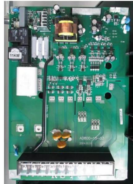
Power board of AD800, 7.5kw
