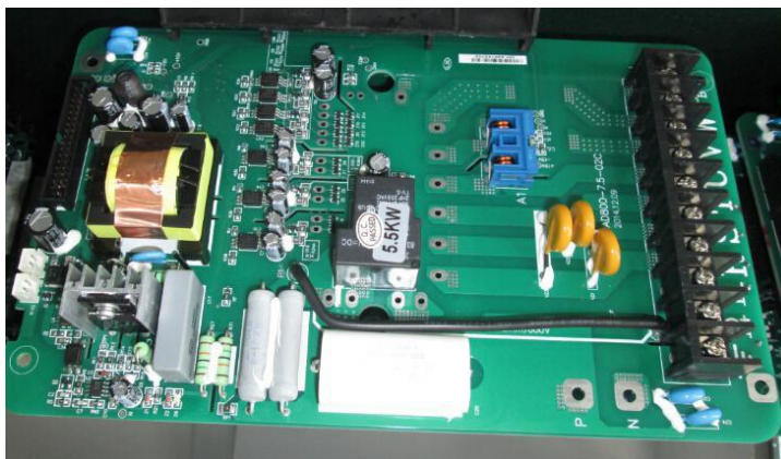
5.5kw power board of AD800's
